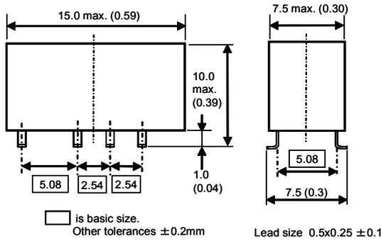
Minimum footprint/ Double coil latch type
