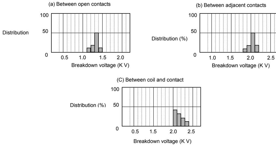
□ ALTERNATION OF VOLTAGE IN DENSE MOUNTING (Magnetic interference)
